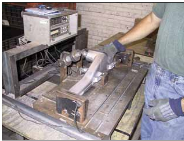
Leak testing determines whether air can penetrate through the casting wall.
