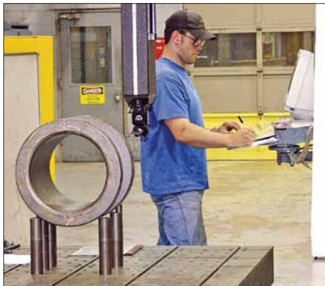
Installing coordinate measuring machines, which verify the dimensional accuracy of castings, is a simple start to performing nondestructive testing.
